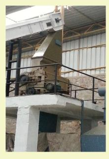
The cake conveyed from Oil Mill is broken to small pieces by a Cake Breaker consisting of spiked rolls made of special alloy.
